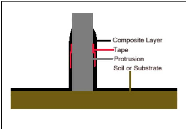
**FIGURE 3 PROTRUSION TERMINATIONS**
